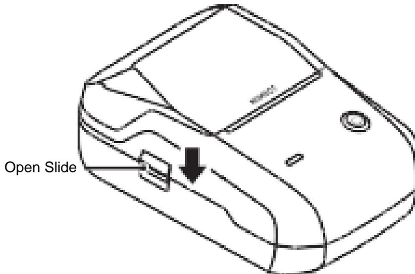
Press the Open Slide on the left to open the paper compartment.
