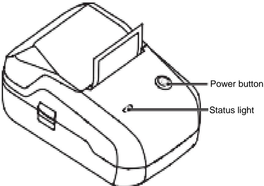
Close the paper compartment and long-press the Power Button to turn the printer on. The sticker will reset the printing position.
