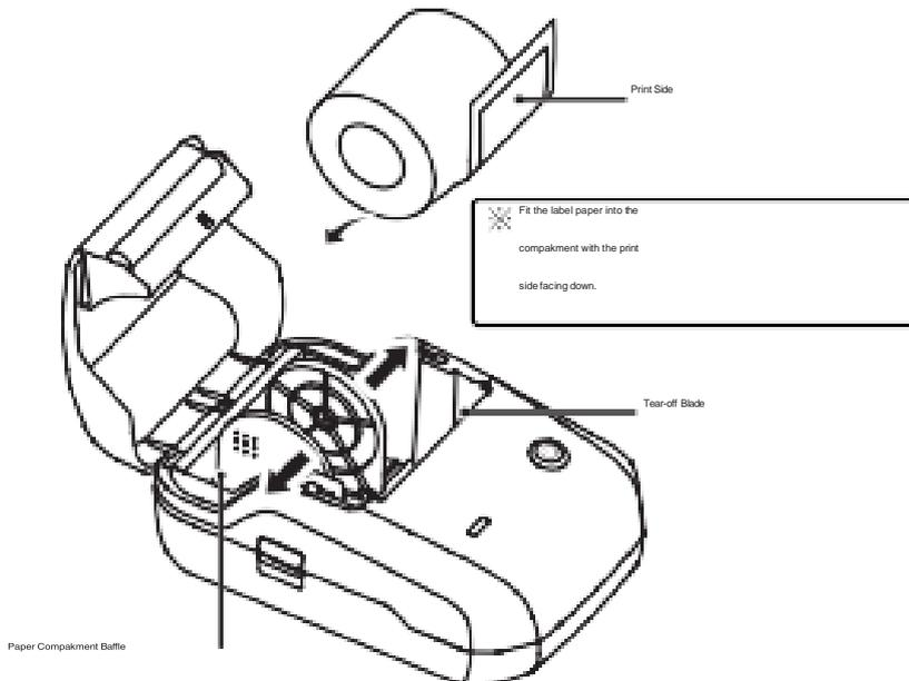
Push the paper compartment baffle to the sides and fit the label paper into the paper compartment with the print side facing down.
